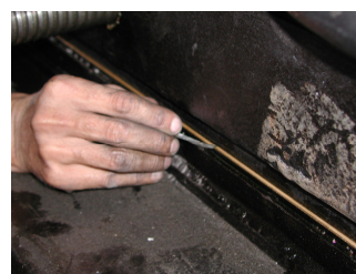
BW1: Wedge locking screw
