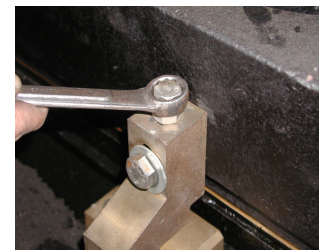
TW2: Adjusting screw
