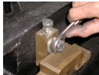
BW1: Wedge locking screw
